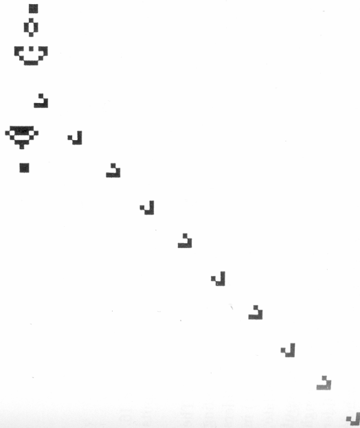
FIGURE 16 A Glider Gun, a periodic LIFE configuration which produces a steady stream of gliders.
